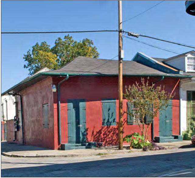
This simple stucco box has deep overhangs at the eaves. Windows and doors are understated and protected by shutters with strap hinges.
