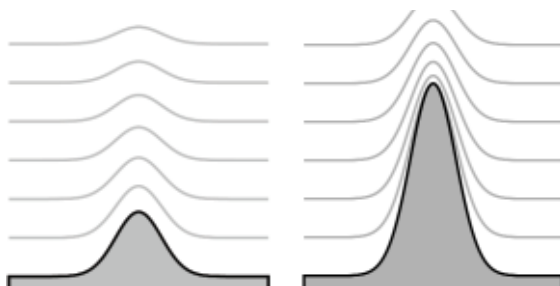
Diffusion Instability. Bumps attract diffusing particles, which follow the gradient of a certain potential field. As it grows, the gradient increases, so a bump grows unstably.
