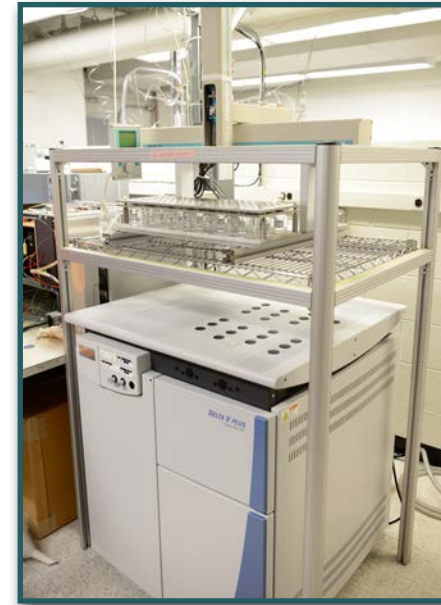
A stable isotope mass spectrometer in Prof. Bess Ward's Guyot Hall laboratory.
